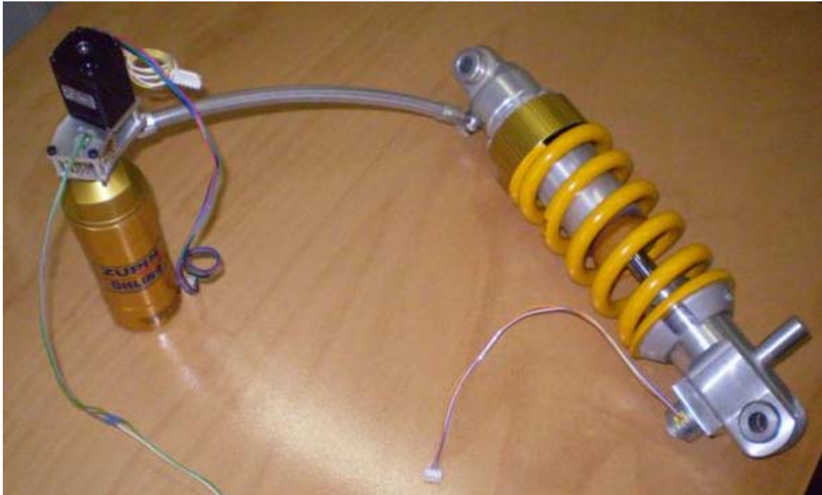
Figure 5: Front shock absorber modified
